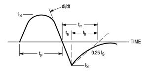
Figure 14. Diode Reverse Recovery Waveform
