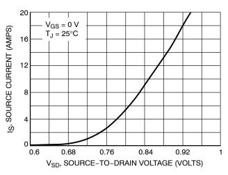
Figure 10. Diode Forward Voltage versus Current
